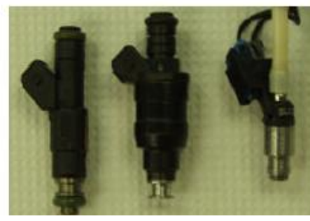
SI multipoint/single-point injection
